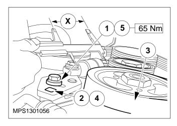
Belt – Power Steering – Pump Drive – Install (13 424 0)
