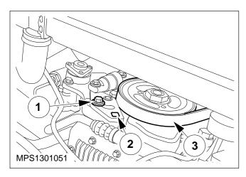
Belt – Power Steering – Pump Drive – Remove (13 424 0)
