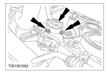
7. Remove the power steering pump.
