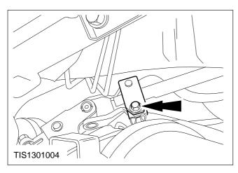
3. Remove the clamp plate bolt securing the flexible coupling to the steering column shaft.
