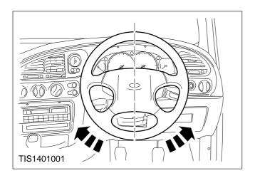
6. Centralise the steering wheel and lock in position.
