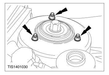
12. Remove the suspension unit and spindle carrier as one assembly.
