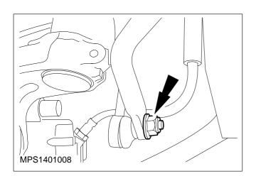
9. Remove the link assembly from the stabiliser bar.
