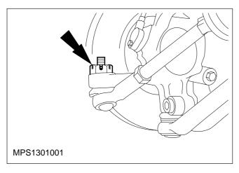
7. Remove the split pin and castellated nut from the steering track rod end.
