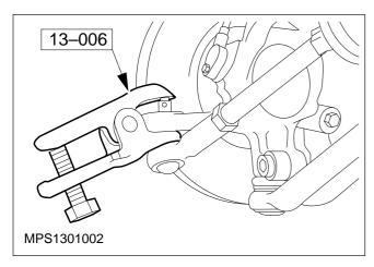
**NOTE:** When the track rod end is separated from the spindle carrier, the ball joint seal should be protected at all times by wrapping in a cloth.
