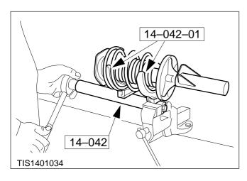
**WARNING:** During this operation the spring is under extreme load, therefore care must be taken at all times.
