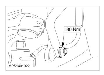
25. Refit the link assembly to the stabiliser bar.
