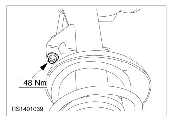
22. Refit the link assembly to the suspension unit.
