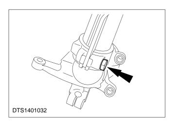
14. Remove the spindle carrier to suspension unit pinch bolt and nut.
