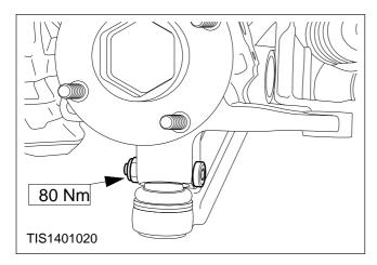
24. Refit the lower arm to the spindle carrier.
