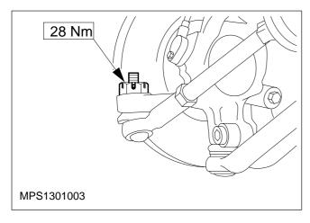
26. Refit the track rod end ball joint to the spindle carrier.
