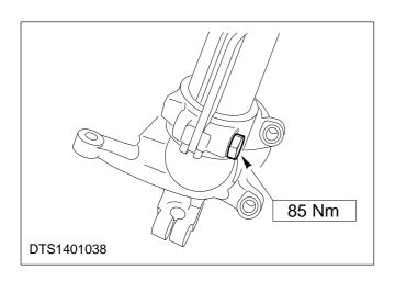
21. Refit the spindle carrier to the suspension unit.
