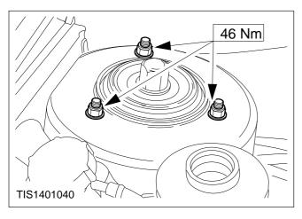
23. Refit the suspension unit and spindle carrier as one assembly.
