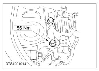
30. Refit the brake caliper assembly.
