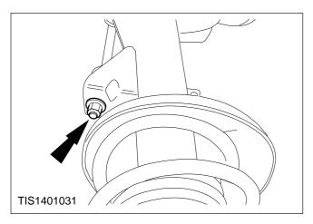
13. Remove the link assembly from the suspension unit.
