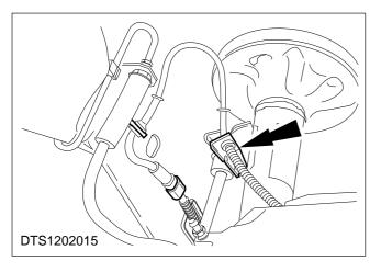
6. Release the ABS sensor lead from the suspension unit.
