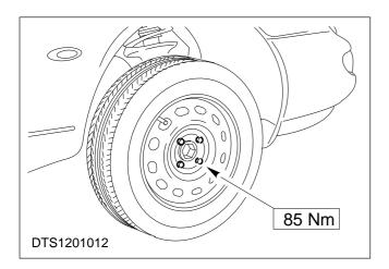
4. Refit the front wheel and lower the vehicle.
