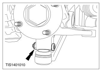
**NOTE:** When the lower arm is separated from the spindle carrier, the ball joint seal should be protected at all times by wrapping in a cloth.
