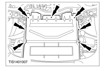
2. Remove the engine lower cover.
