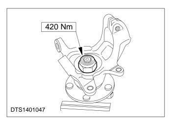
11. Refit the hub retaining nut.
