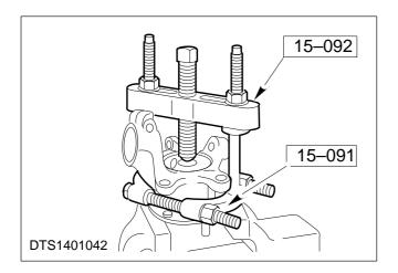
**NOTE:** When the hub assembly is disengaged from the spindle carrier the bearing will be damaged and will need to be renewed.
