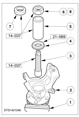
**NOTE:** Rotate the spindle carrier during this operation to ensure correct seating.
