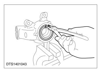
3. Remove the inner and outer snap rings, (outer ring shown).
