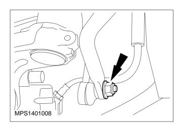
6. Disconnect the stabiliser bar to suspension link assembles.
