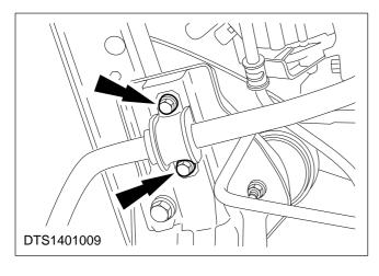
7. Remove the stabiliser bar.
