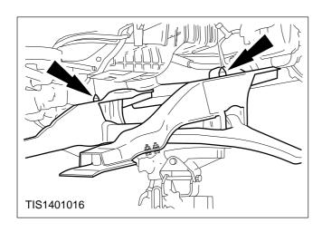
16. Raise the crossmember engaging the guide pins into the alignment holes.
