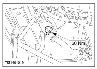
19. Refit the engine mount securing nuts.
