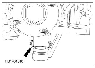
**NOTE:** When the lower arm is separated from the spindle carrier, the ball joint seals should be protected at all times by wrapping in a cloth.
