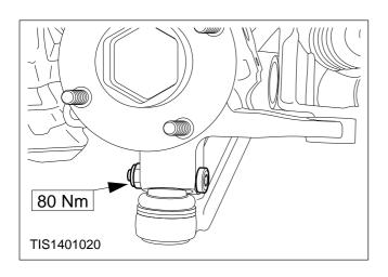
20. Refit the lower arm ball joints to the spindle carriers.
