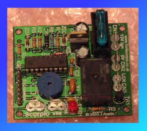
The Lock on Go unit, is specifically designed for the Ford Scorpio 95+, but may be suitable for other vehicles. It provides added security, in that all the doors are locked after a preset speed is reached. This can protect against opportunist crimes, such as theft of handbags, briefcases etc from the passenger or back seat. Also it makes attempts to steal your car more difficult, for carjacking criminals. The unit is straight forward to fit and requires four wires
